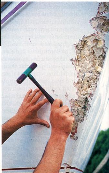
Tapping a hull with a hammer was a surveying technique in the days of wooden boats, but the practice remains essential today when inspecting fiberglass vessels for core saturation, resin starvation, and delamination.
