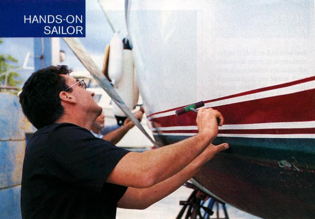
Tapping a hull with a hammer was a surveying technique in the days of wooden boats, but the practice remains essential today when inspecting fiberglass vessels for core saturation, resin starvation, and delamination.
